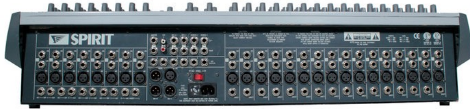
Back of a mixer where input and output cables are patched.
